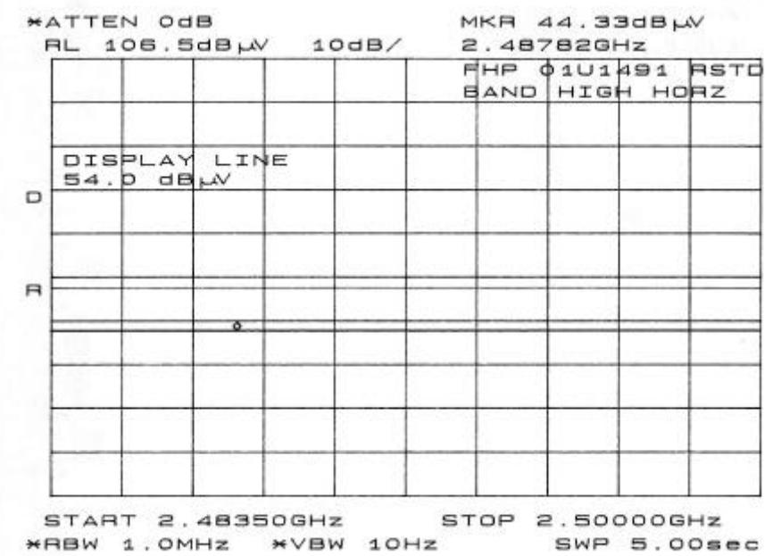
**15 dBi OMNI ANTENNA - SPURIOUS RADIATED EMISSIONS**
