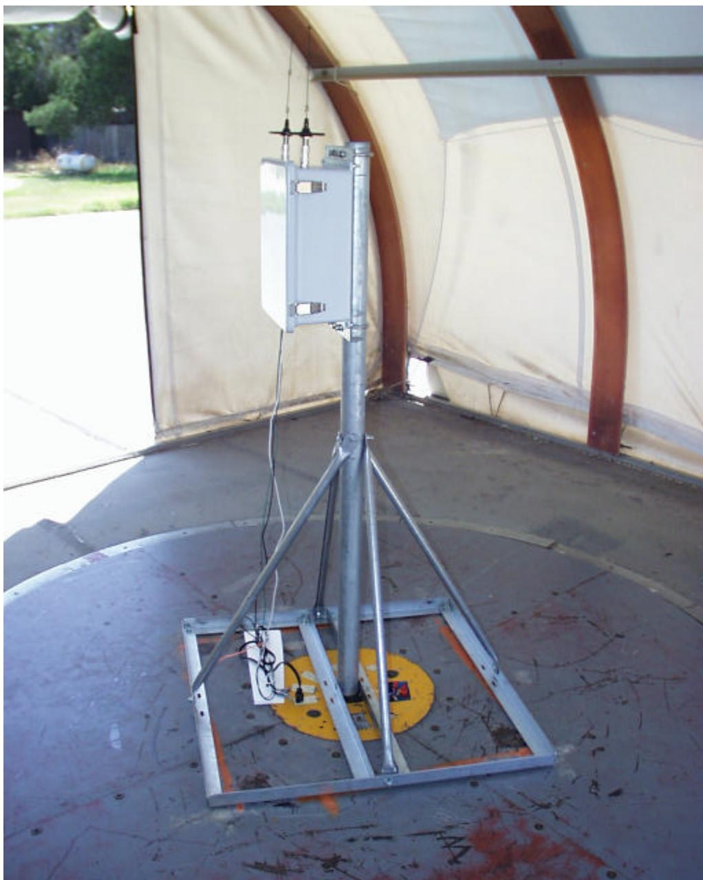
**DIGITAL DEVICE RADIATED EMISSIONS MEASUREMENT SETUP FOR POWER OVER ETHERNET**
