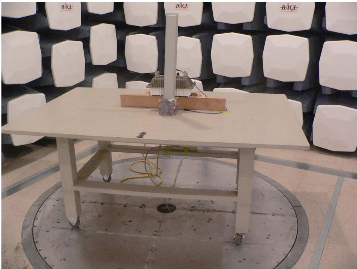
POWERLINE CONDUCTED EMISSIONS MEASUREMENT SETUP
