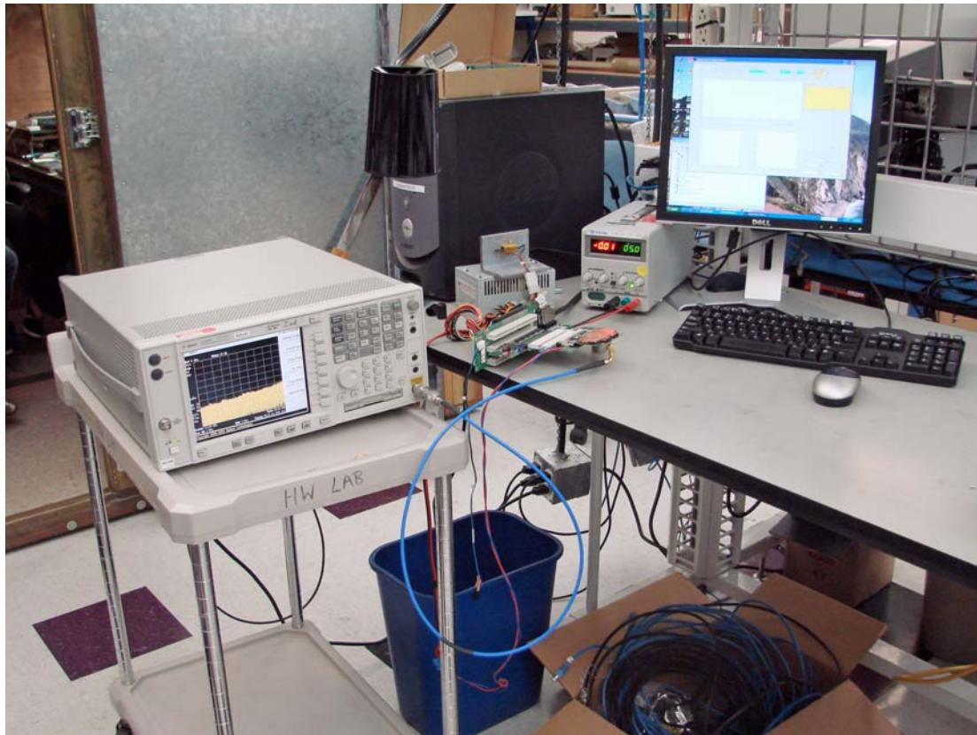
**RADIATED RF MEASUREMENT SETUP**
