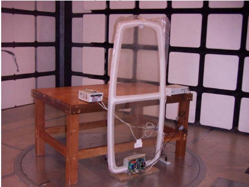
**AC MAINS LINE CONDUCTED EMISSION (0.15-30 MHz)**
