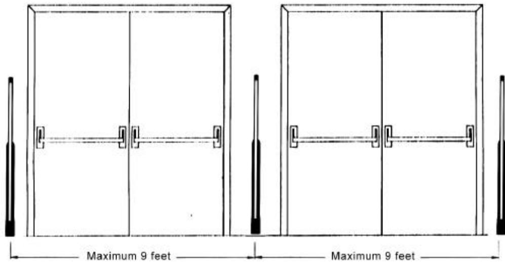
This type of installation consists of one receiver and two transmitters. Installing the receiver in middle and the transmitters at the ends. Each transmitter post will be connected to the receiver post. The Multi-Guard system uses an interconnection cable from the transmitter to the receiver. The gates are mounted on both sides of the opening and cover a maximum distance of 18 feet (when using our Supersensor or Super Pencil tag)
