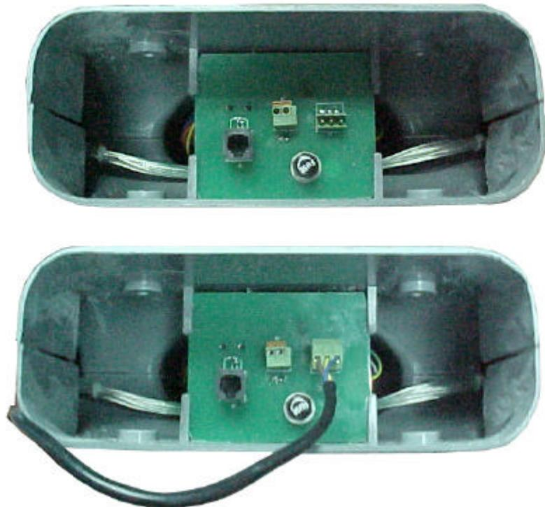
Connect the interconnection cable in to the RJ45 socket on PC Board as the picture shows, (both transmitter and receiver)
