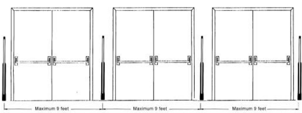
Then the wider the opening, the more systems are needed. This type of installation consists of two-transmitters and two-receiver pedestal with interconnection from the transmitter to the receiver. The gates are mounted on both sides of the opening and cover a maximum distance of 27 feet. (When using our Supersensor or Super Pencil tag)
