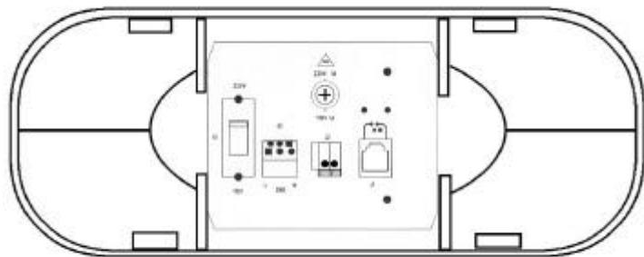
When using a slave post, connect the interconnection cable into the RJ45 socket on PC Board
