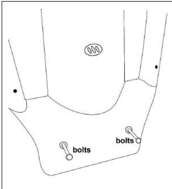
Use the tool provided to screw down the nuts
