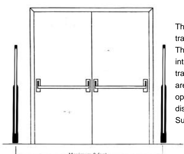
This type of installation consists of one transmitter and one receiver pedestal. The Multi-Guard system uses an interconnection cable from the transmitter to the receiver. The gates are mounted on both sides of the opening and cover a maximum distance of 9 feet (when using our Supersensor or Super Pencil tag)
