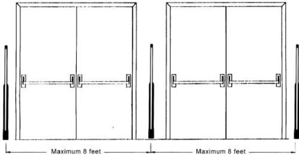
This type of installation consists of one master Mono-Guard system and two slaves with the master in middle and the slaves at the ends. Every gate-to-gate distance is both 8 feet maximum; the three gates will cover a maximum distance of 16 feet. Each slave post will be connected to master post.
