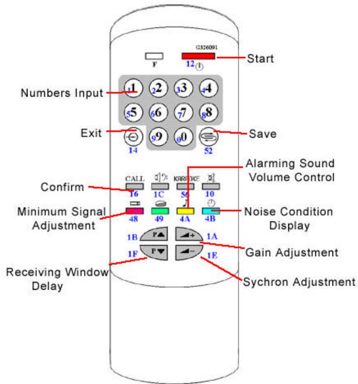
Usually, the most frequently used function is to adjust the Minimum Signal Adjustment figures, (see entry H). The smaller the figure is, the more sensitive the system is while the more vulnerable to false alarms. Properly tuning this figure to ensure the system works at the certain distance at best sensitivity and with minimum false alarms.
