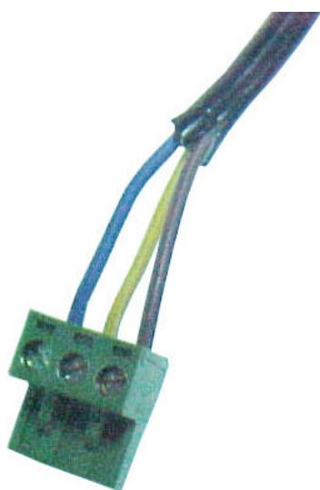
Put the plug to face towards you with the side where there are metal screws. Connect the N line to left terminal, the L line to right terminal, and the ground line to middle terminal.
