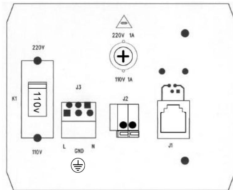
There are two external alarm outputs. First press down the yellow button, then insert the external alarm wire into the wire holding hole and release the yellow button, the wire will be fixed onto the system. Each external alarm output has a contact rating of 1A/220VAC
