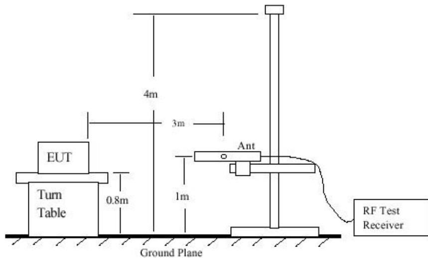
Fig 1: Radiated Emission Measurement 30 to 1000 MHz
