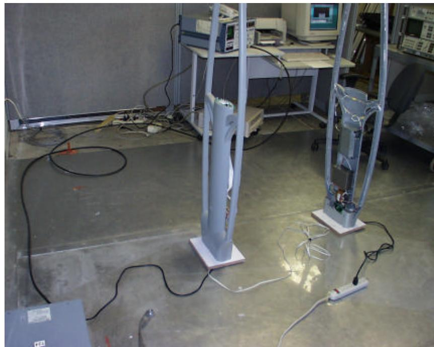
Multi-Guard Conducted Emission Setup
