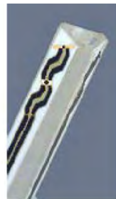
Figure 2.3 Probe Thick-Film Technique
