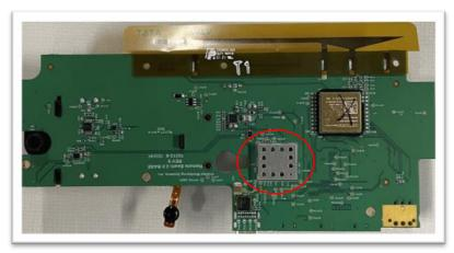
With Shield Can Installed (Bottom)
