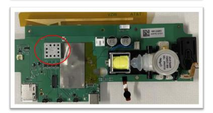
With Shield Can Installed (Top)
