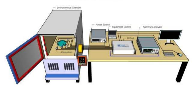
A full system calibration was performed on the test station and any resulting system losses (or gains) were considered in the production of all final measurement data.
