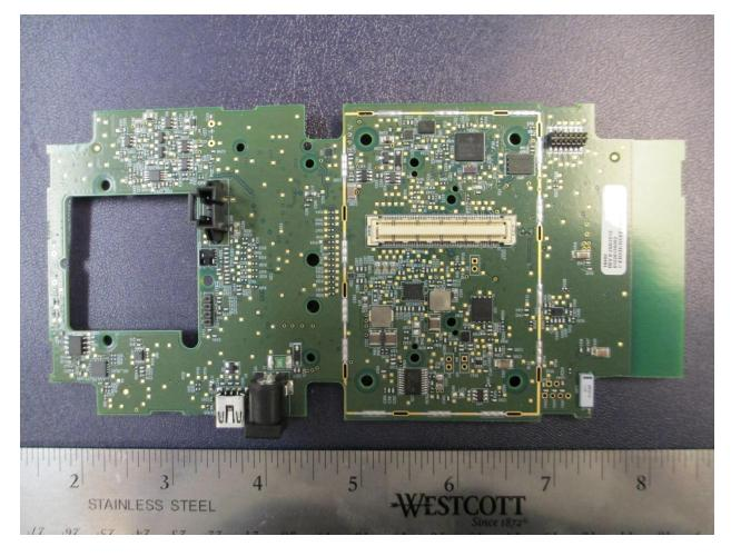
Main Board Bottom View without Processor Board
