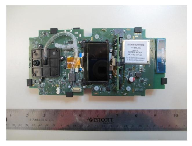
Main Board Top View With Camera Board and Display
