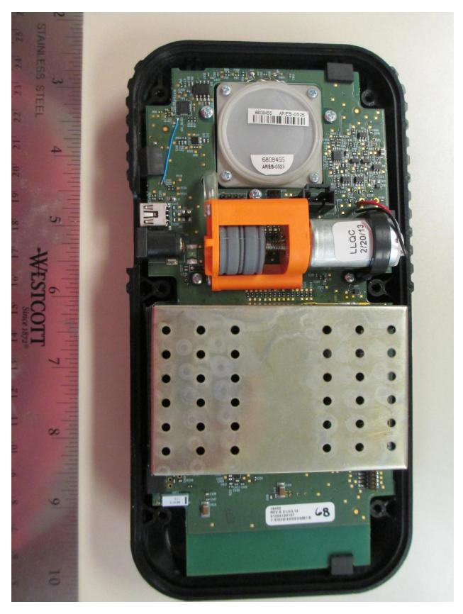
PCBs Inside Remote Breath Housing With Back Removed
