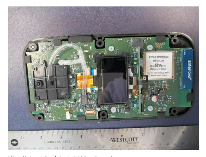
PCBs Inside Remote Breath Housing With Front Removed
