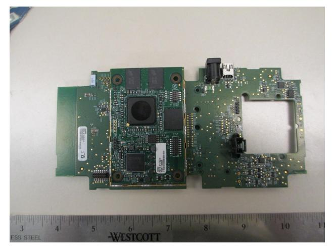
Main Board with Processor Board Attached
