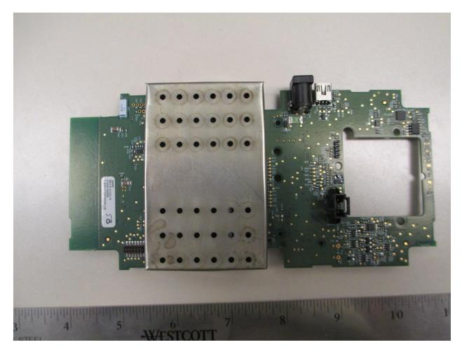
Main Board with Shield Can Over Processor Board
