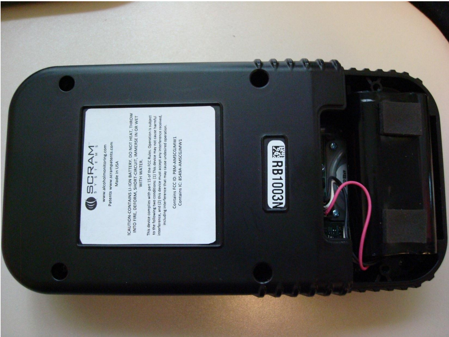
Remote Breath Back w/ Battery Cover Removed
