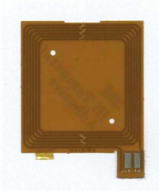
**13.16 EUT Internal – GSM 850/1900 Antenna**
