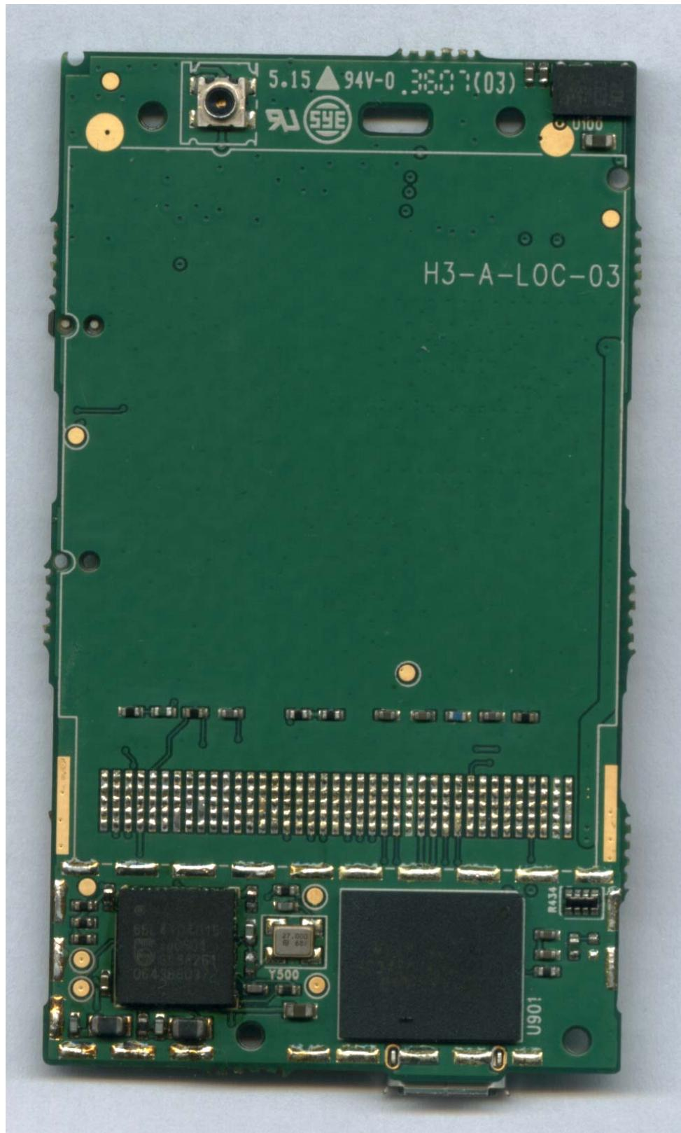
**13.13 EUT Internal – PCB Side two**
