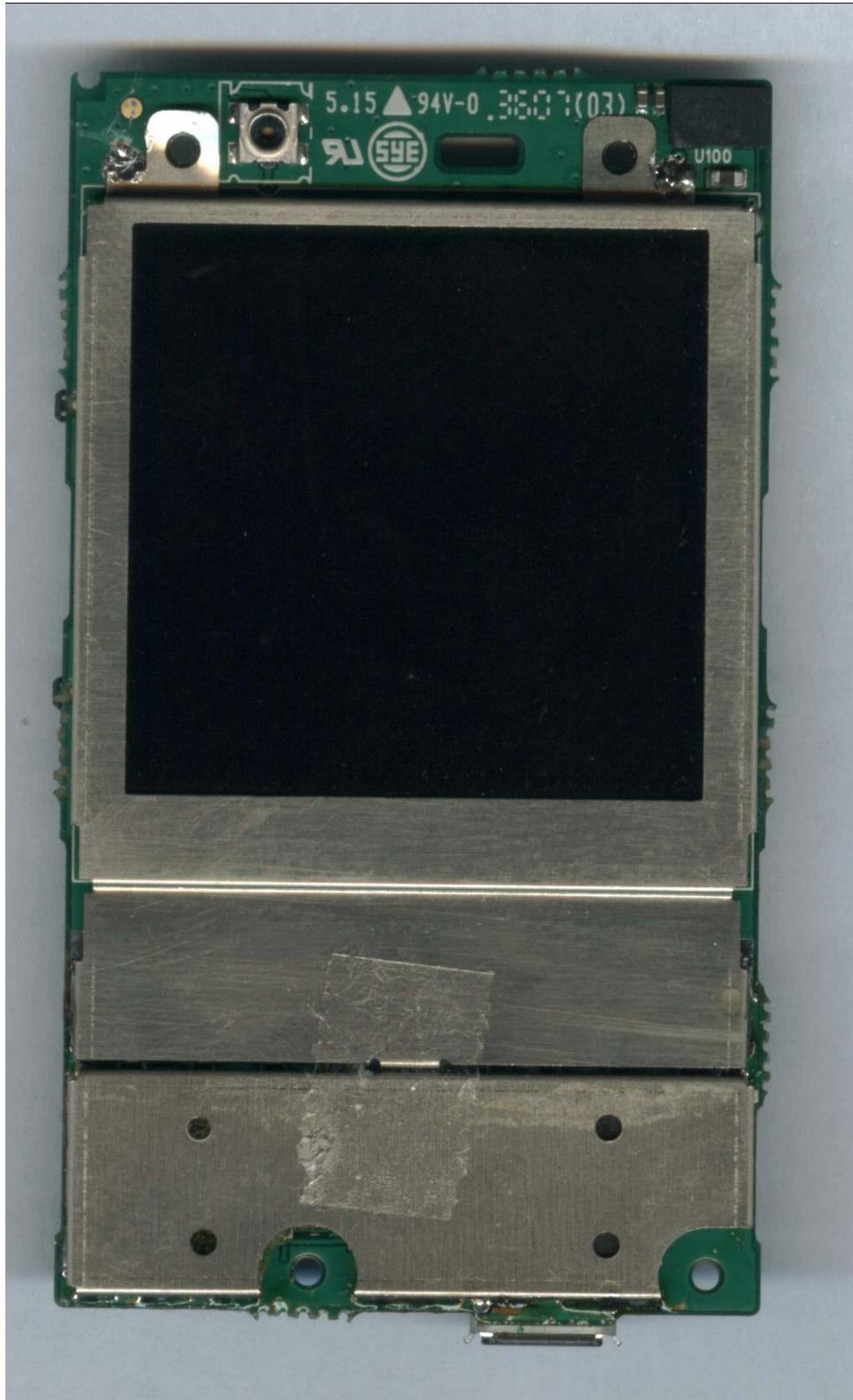
**13.12 EUT Internal – PCB Side one, LCD and RF Sheilding Removed**
