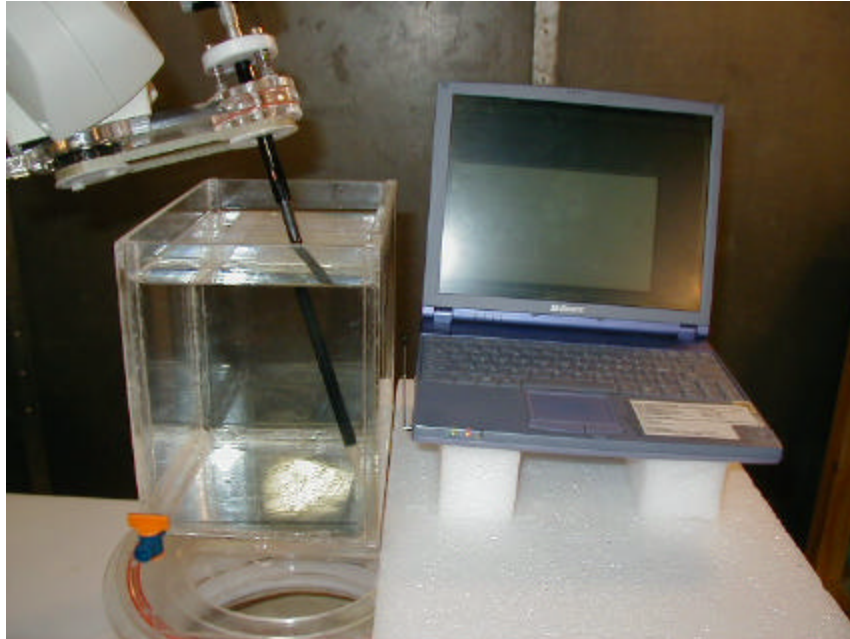
Figure S2. Configuration 1 per Table 9 (Antenna separated from box phantom by 15 mm)
