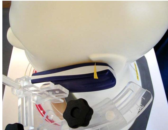
It is also important to check that the front face of the phone sits squarely against the platform of the flattened ear and is not raised more at one side than the other.
