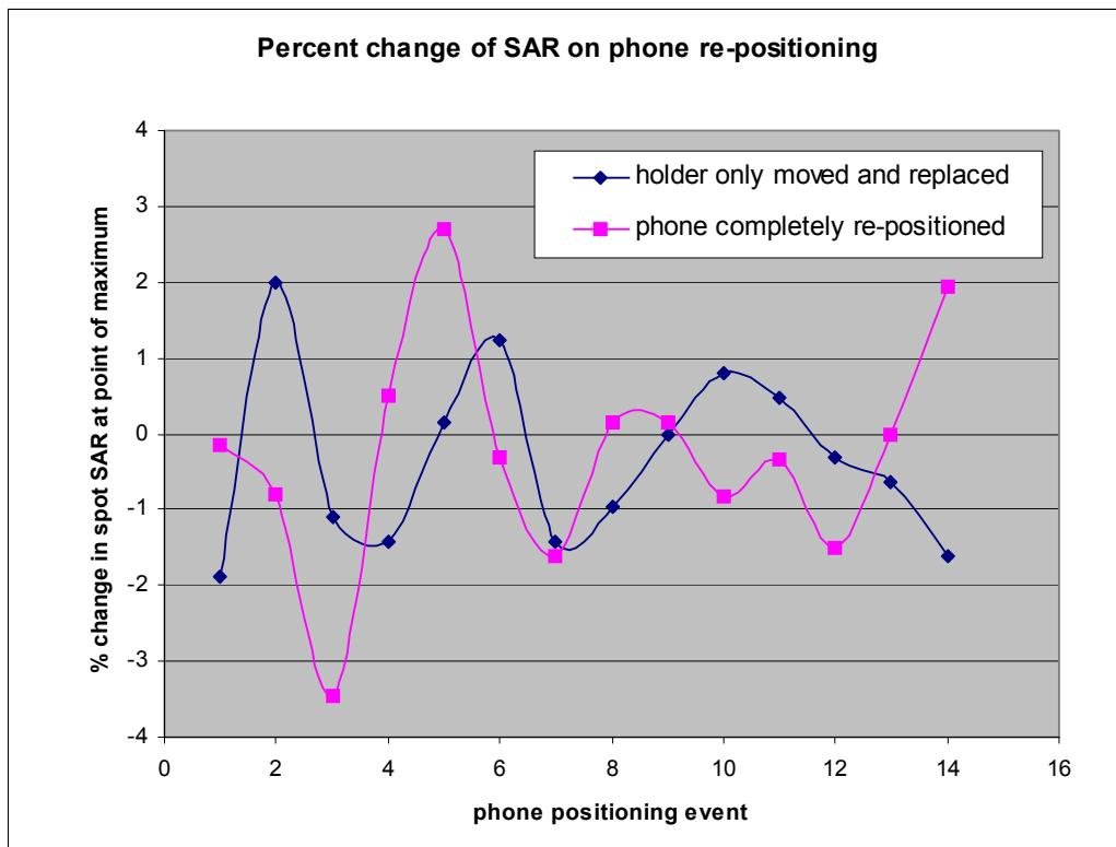
The graph suggests that an uncertainty of +/- 2% occurs when the phone holder is moved away and then replaced, whilst a higher uncertainty of +/- 3% is associated with complete repositioning of the phone.
