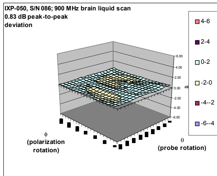
Comparison of the measurements confirms that the isotropy is not significantly different for brain and body fluids.
