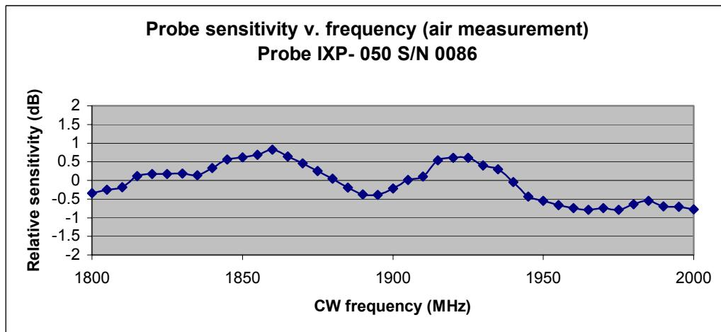
Whilst the measurements indicate a variation of 1.6dB over the range 1800 to 2000MHz, the response at 1800 and 1900MHz is very similar. This is borne out for probes calibrated in liquid at both 1800MHz and 1900MHz, where the probe calibration factors are similar.
