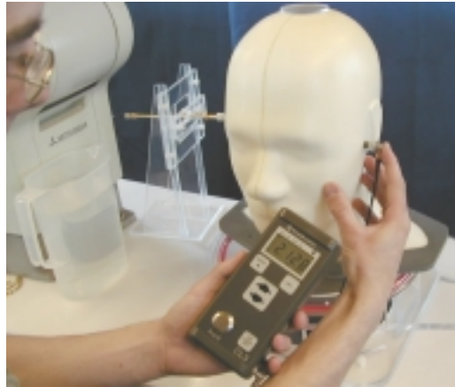
Figure 3: Showing an ultrasonic thickness measurement being performed
