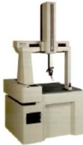
Figure 1: Mitutoyo co-ordinate measurement machine (Model C574)
