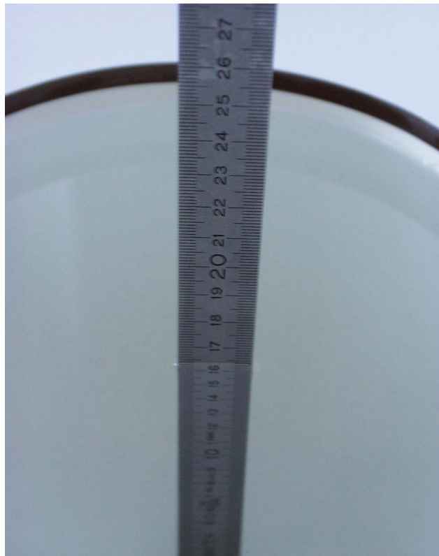
Fig. 22: Liquid depth for PCS 1900 head measurements (16.4 cm).
