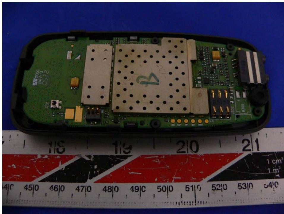
**EUT Component with Shielding View**
