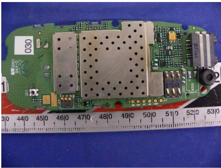
**EUT Component without Shielding View**
