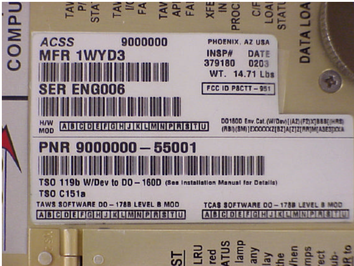
Figure 3: Unit Front Name Plate
