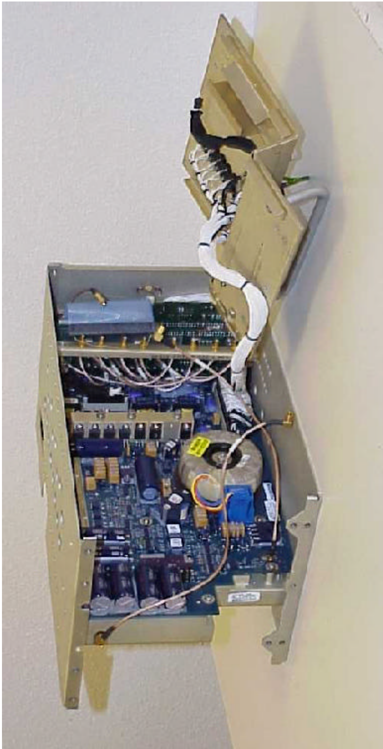
Figure 12: View of Unit Side, A5 Receiver and Front Panel Removed, Showing A4 Power Supply/Modulator Assembly
