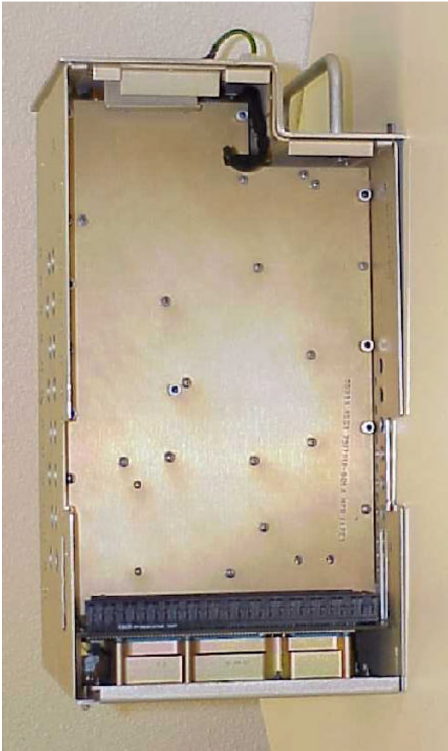
Figure 11: View of Unit Side with A2 Processor Removed Showing A3 Transmitter Assembly With Cover
