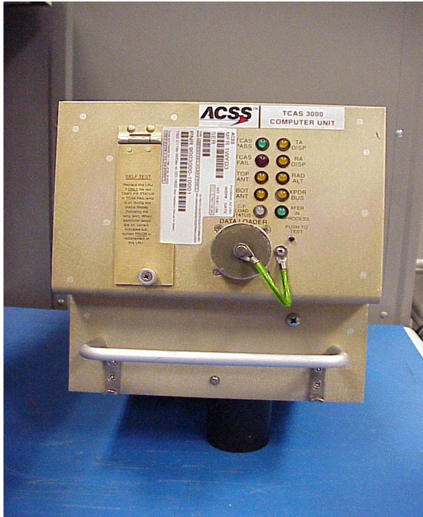
Figure 14: 6 MCU Unit Front Name Plate
