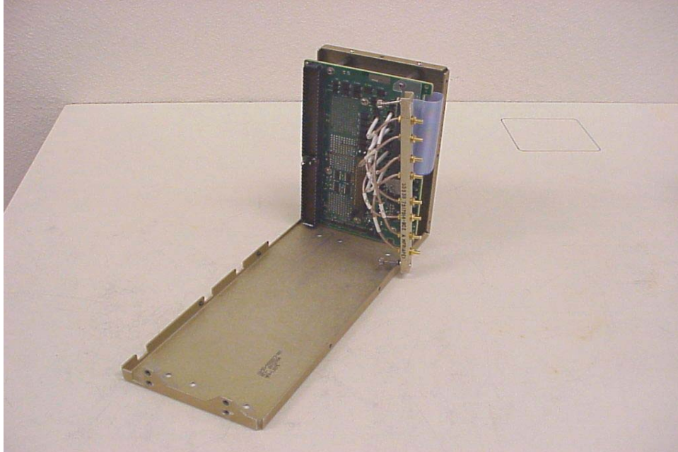
Figure 13: View of 4 MCU Unit, Showing A1 Interconnect Assembly
