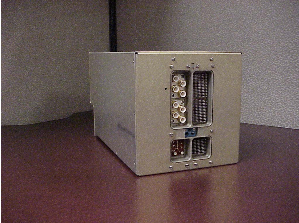
Figure 5-2: Back Panel Showing ARINC Connector
