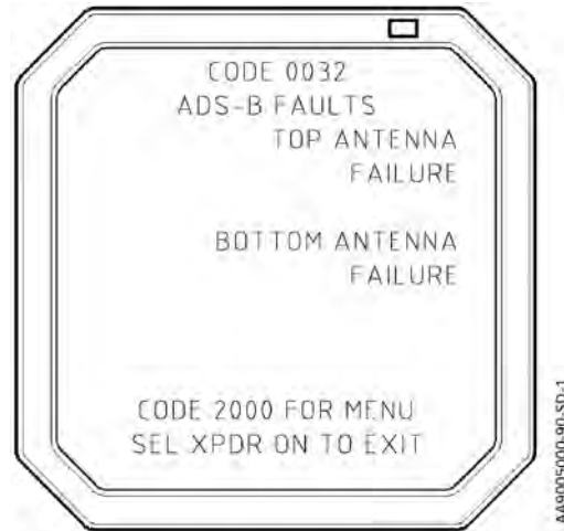
Figure 6-20: ADS-B Fault Page 3 (Code 0032)
