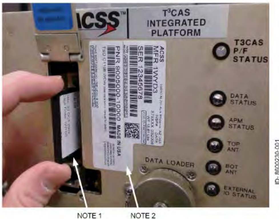
Figure 5-5: Compact Flash Card Access Port and LRU Identification Label
