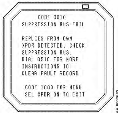
Figure 6-11: Suppression Bus Fail Page
