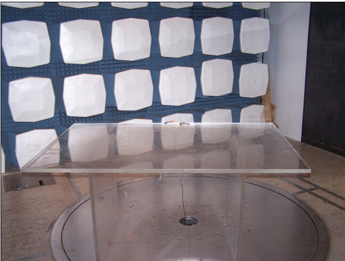
Photograph 2. Radiated Emission Test Setup
