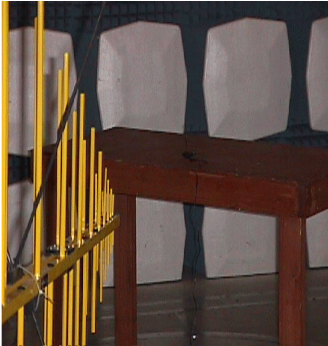
Figure 2: Test Setup Photo for Intentional Radiator - Radiated Emissions, Occupied Bandwidth, RF Power Output, and Peak and Average Measurements
