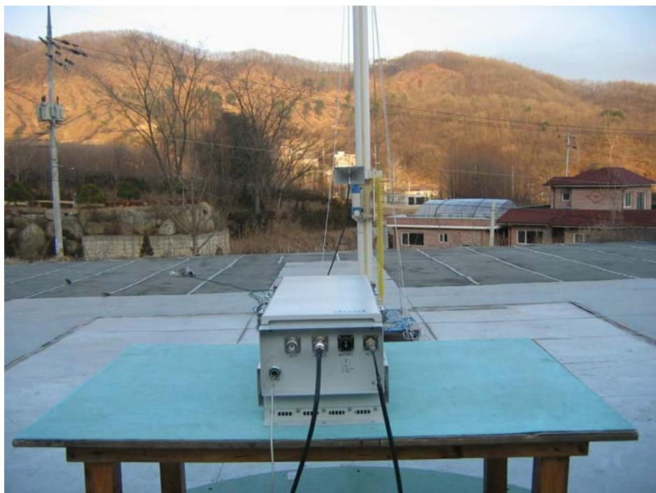
**Radiated Emission Test Setup(Dornor+Remote)**
