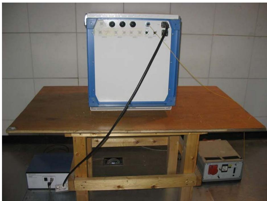
**Power Line Conducted Emission Test Setup(Remote)**
