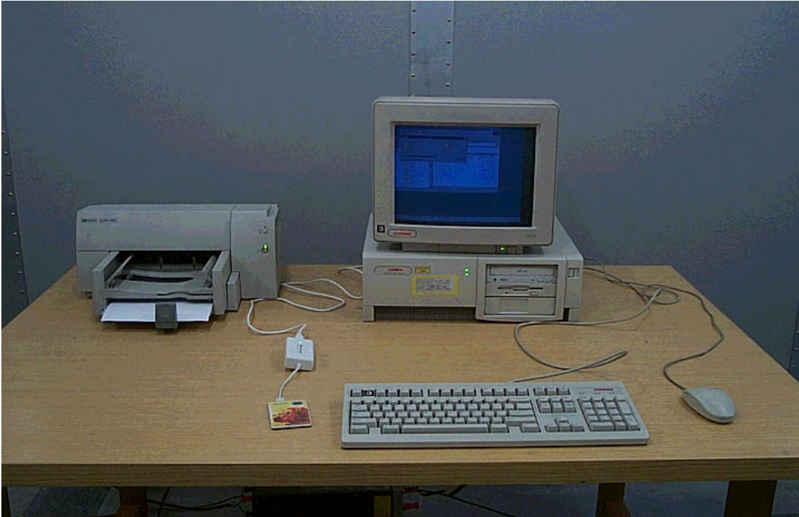
Photograph 1 : Setup for Conducted Emissions
