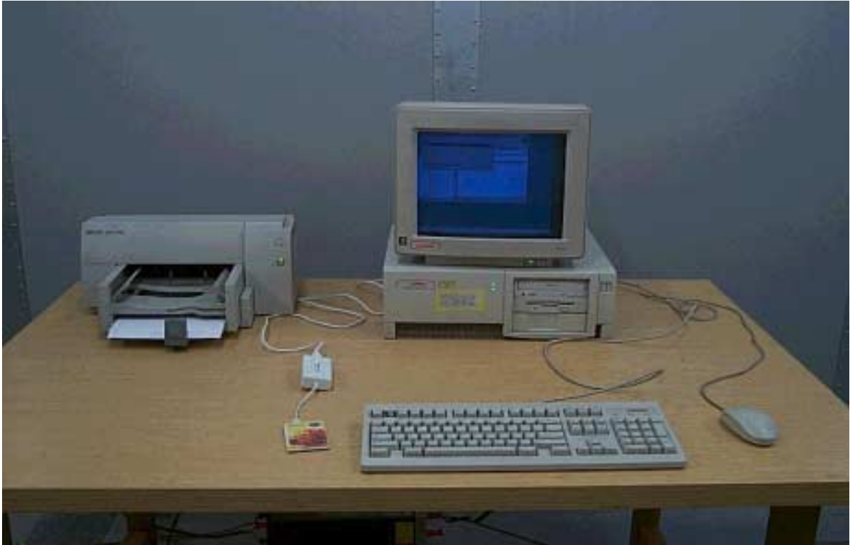
Photograph 1 : Setup for Conducted Emissions
