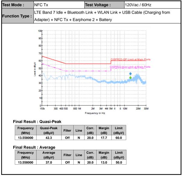
Remark: 13.558MHz is the NFC RF fundamental signal..
