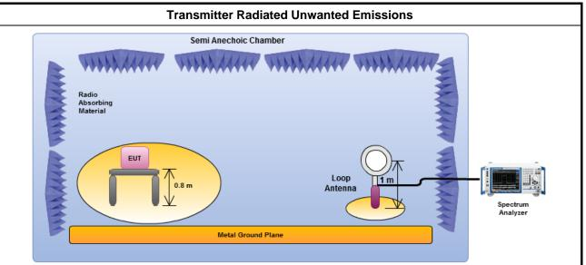
Magnetic field tests shall be performed in the frequency range of 9 kHz to 30 MHz using a calibrated loop antenna. The center of the loop shall be 1 m above the ground. Electric field tests shall be performed in the frequency range of 30 MHz to 1000 MHz using a calibrated bi-log antenna. the antenna height shall be varied from 1 m to 4 m.
