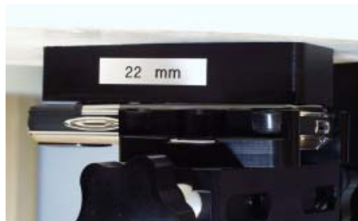
Photo of the device positioned for Body SAR measurement using separation distance. The spacer was removed for the tests.
