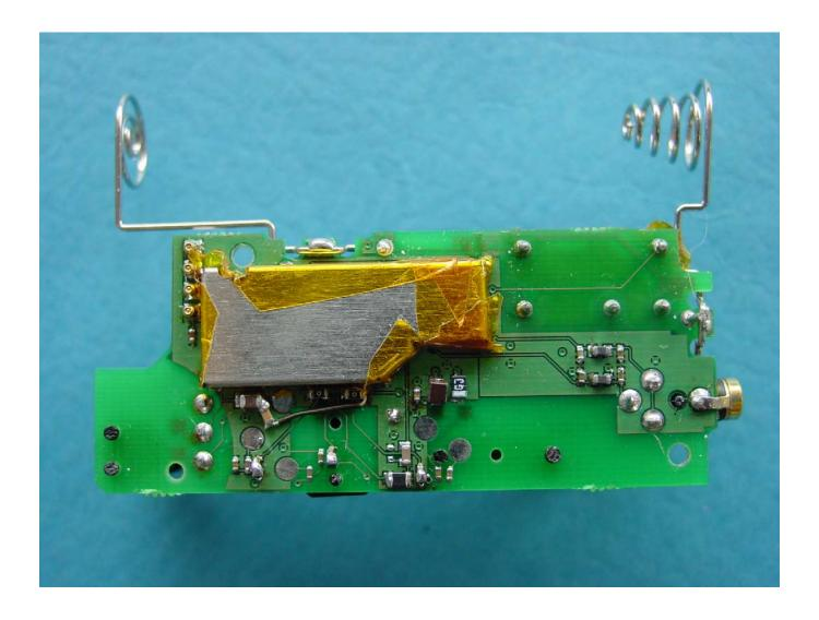
Photo 5. Base unit: Printed circuit board: LibertyLink chip side
