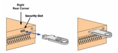
5. Thread the anti-theft device's pin through the bolt's holes, and insert the pin into the main body of the anti-theft device, as described in the documentation that came with your device.
