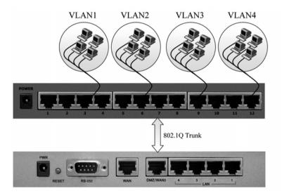
Figure 10: Tag-based VLAN
