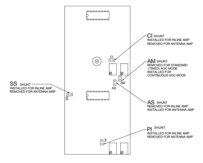
Figure A-1. Autoset Shunt Positions.
