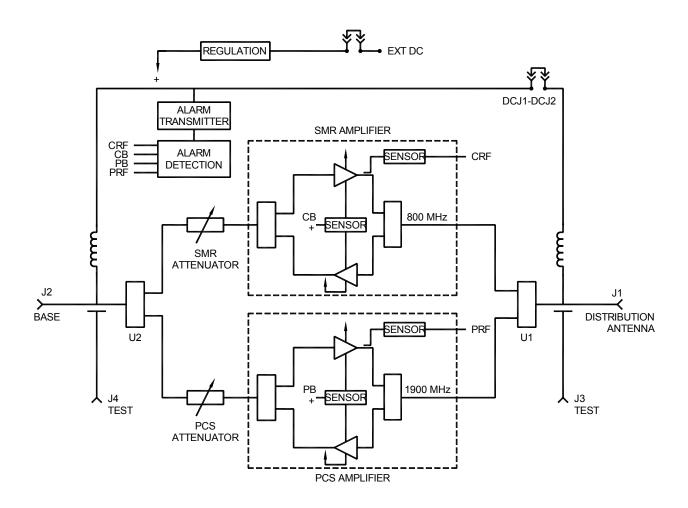
Figure 2-1. A300 Bidirectional Amplifier - Block Diagram
