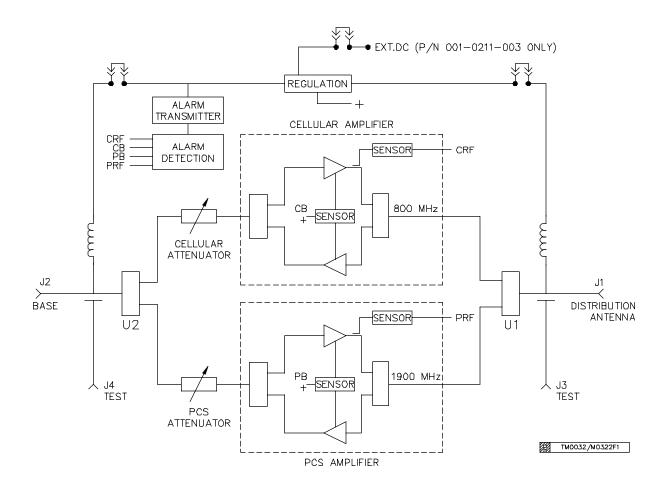
Figure 2-1. A211 Dual Band Bidirectional Amplifier - Block Diagram
