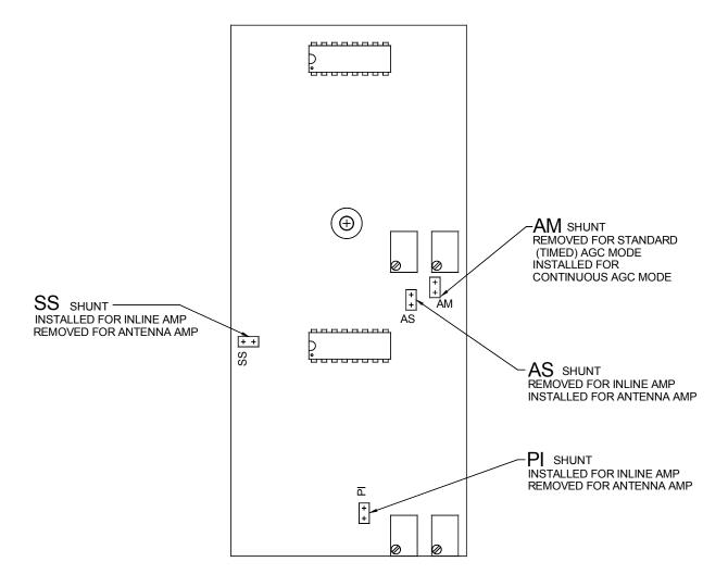
Figure A-1 Autoset Shunt Positions.
