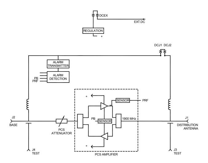
Figure 2-1 A238 Bidirectional Amplifier - Block Diagram
