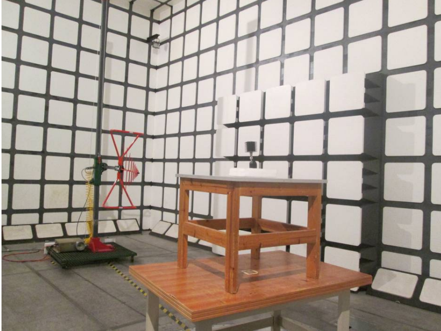
Transmitting Radiated Emissions (Below 1 GHz)
