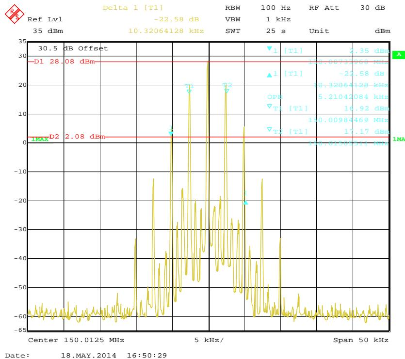
**Emission Mask with High Power**
