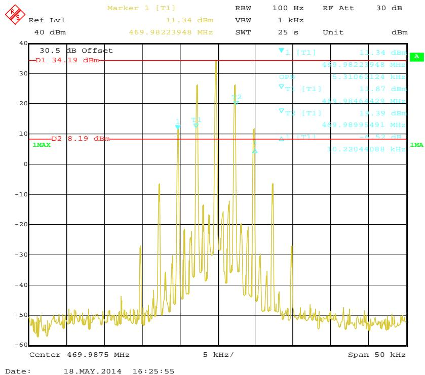
**Emission Mask with High Power**
