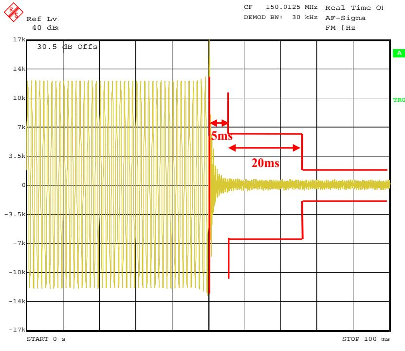
**Analog Modulation 150.0125 MHz, Turn off**
