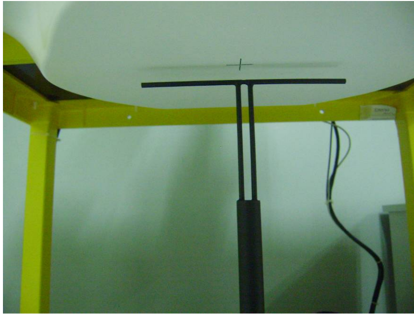
Setup Photo of Dipole Antenna
