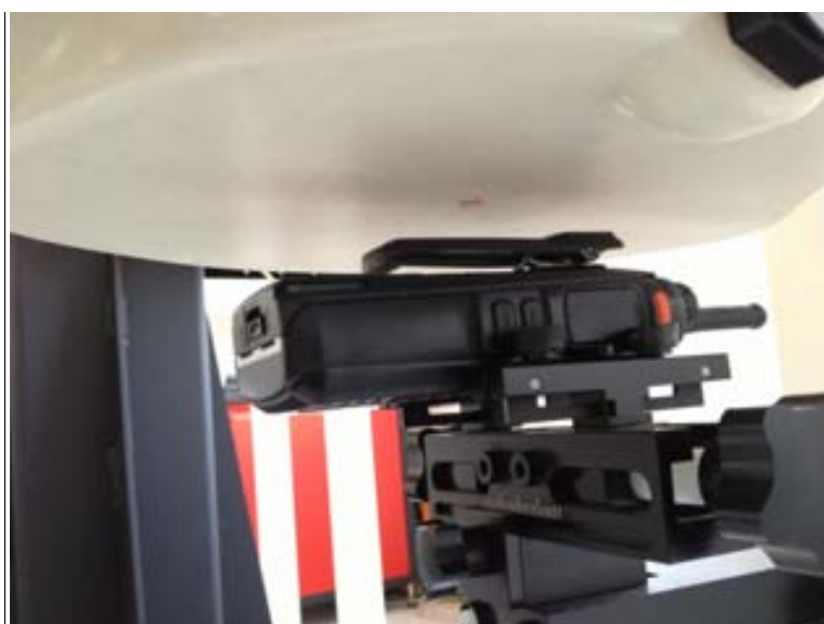
0mm Body-worn, The EUT display towards ground, belt clip attach the phantom
