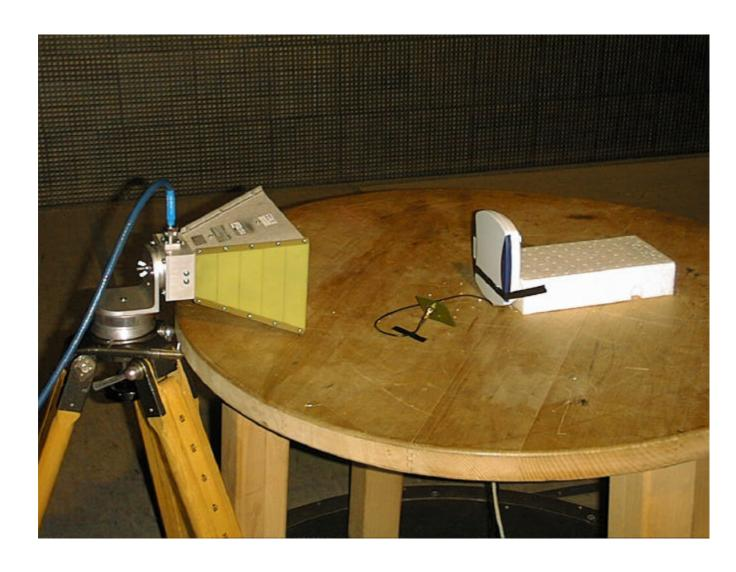
Description: Test setup radiated emissions above 18 GHz\*
