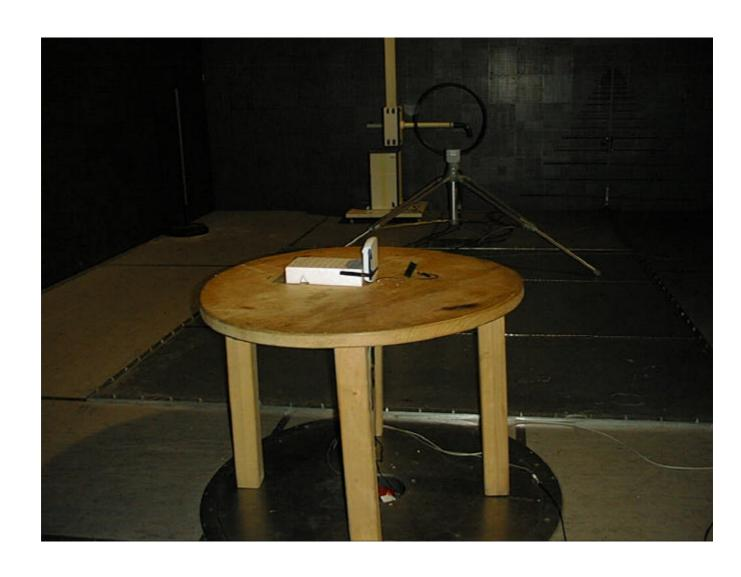
Description: Test setup radiated emissions above 2 GHz\*
