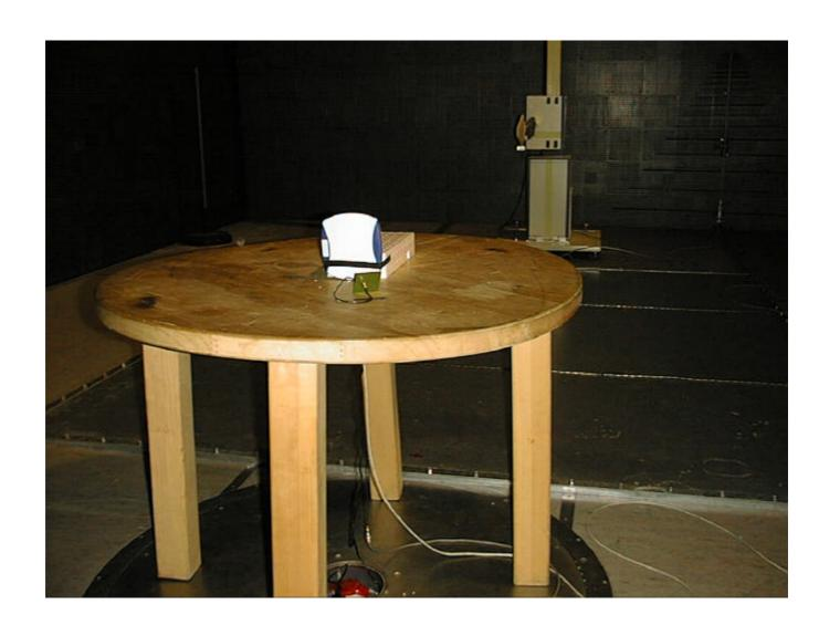
Description: Test setup radiated emissions below 30 MHz
