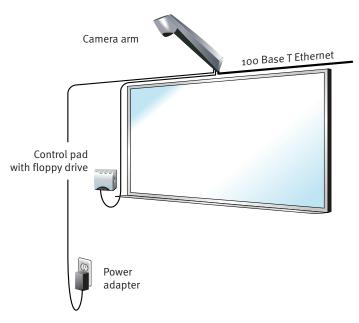
CopyCam wiring can be either:
