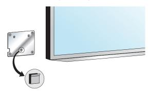
3 Drive the toggle bolt screws (provided) through the mounting plate and toggle bolt, and if a stud was located, drive a #8 x 1.5 inch drywall screw (provided) through the mounting plate and wall into the stud.
