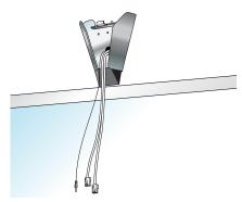
Leave about 24 inches of cable extending from the camera arm mounting plate exit hole for later connection to the camera arm, as shown.
