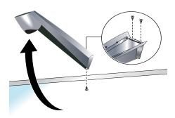
Fasten the arm in place using the three arm-securing screws provided. (The larger screw secures the bottom of the arm.)
