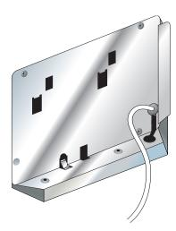
Route the RJ14 cable from the back of the control pad into the wall and up to the camera arm mounting plate exit hole. If necessary use a fish tape to fish the cable end through the wall to the camera arm mounting plate exit hole.
