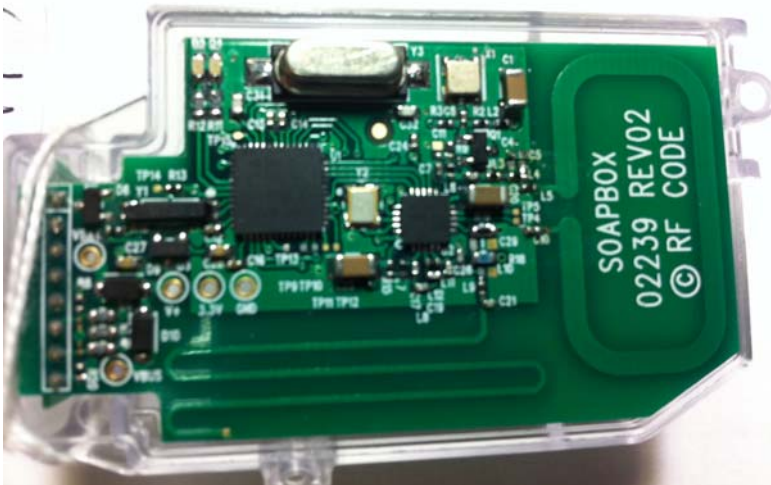
Photograph 8.3.1 – Top View Showing Printed Circuit Antennas
