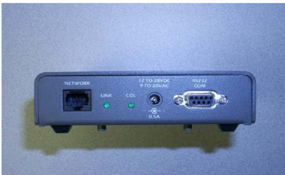
Figure 2.2 – Mantis™ II 433.92 MHz Reader (rear view) showing connections for Network/Ethernet (RJ-45), Power, and Serial/COM (RS-232).
