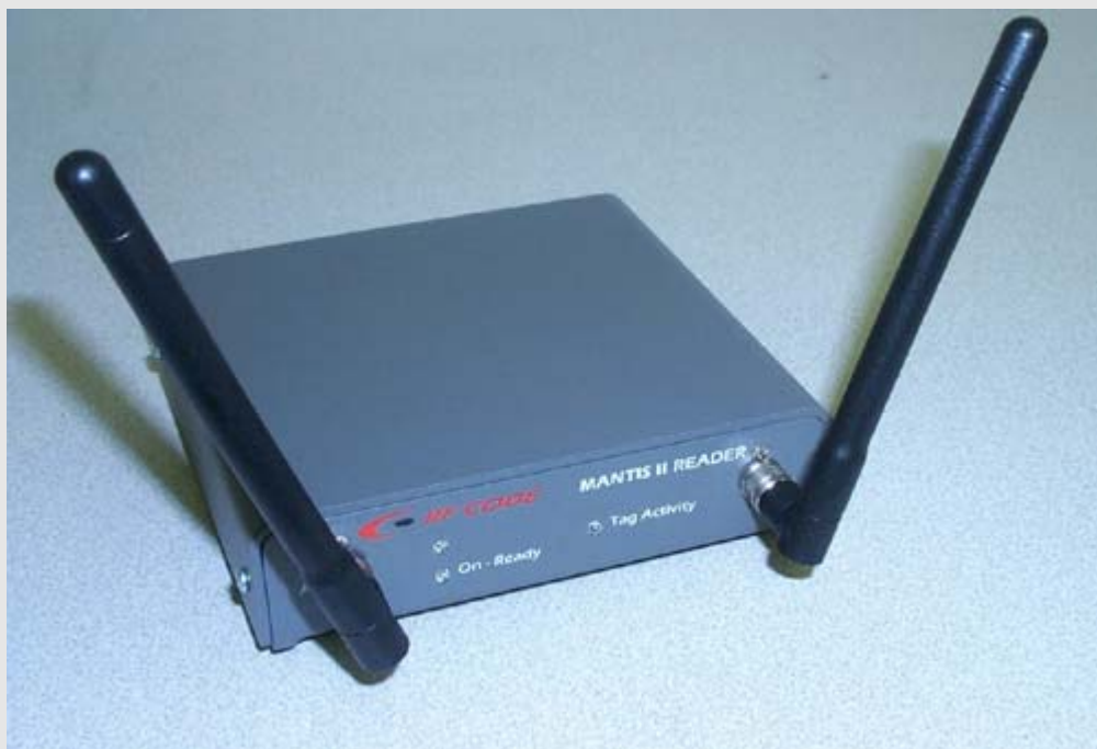
Figure 2.1 – Mantis™ II Reader (front view) shown with standard ¼-wave helical antennas.
