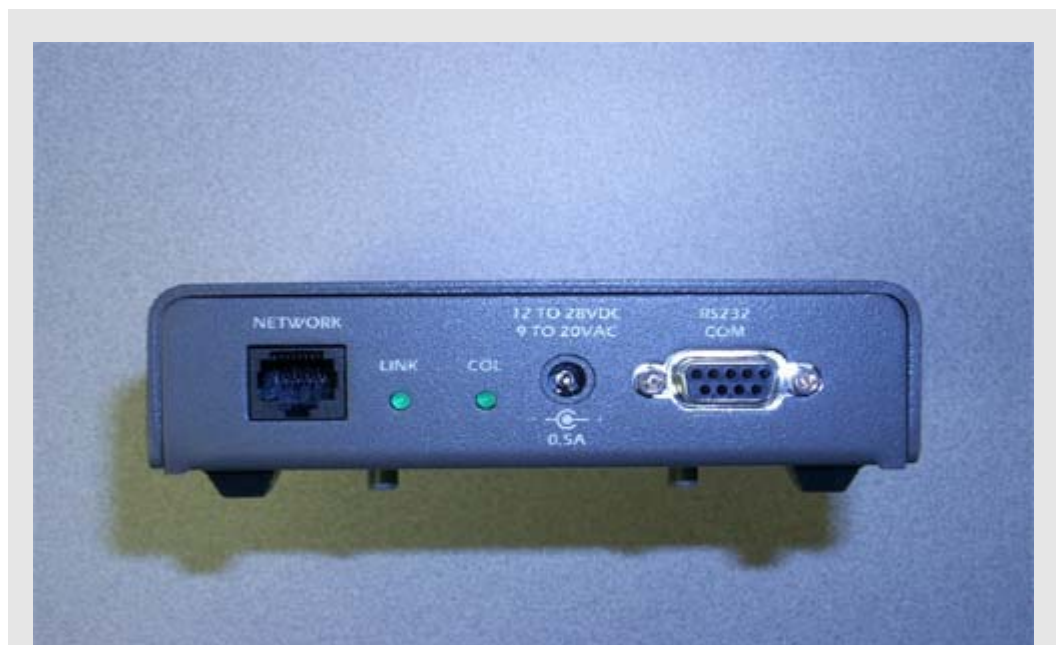
Figure 2.2 – Mantis™ II Reader (rear view) showing connections for Network/Ethernet (RJ-45), Power, and Serial/COM (RS-232).
