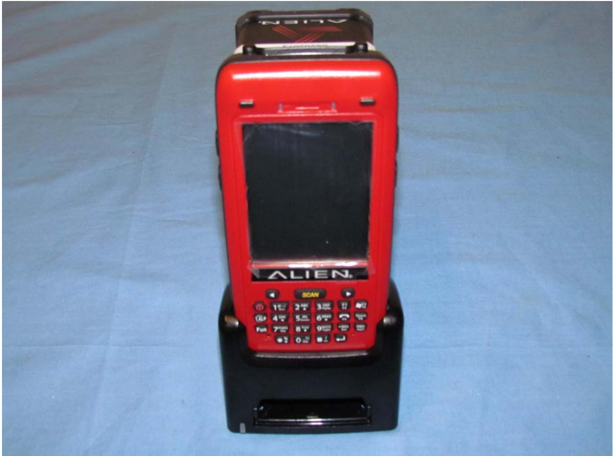
Alien Technology ALH-90XX Handheld RFID Reader installed in Charging Station
