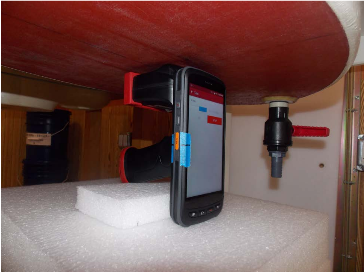
Test Position Top RFID Testing 0 mm Gap
