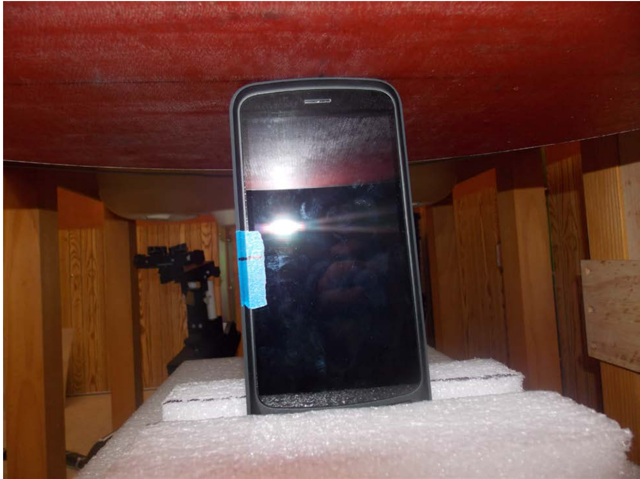
Test Position Top Testing 0 mm Gap
