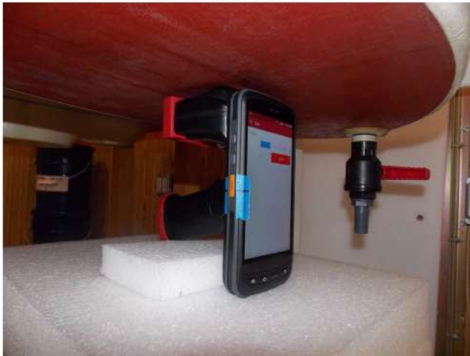
Test Position Top RFID Testing 0 mm Gap
