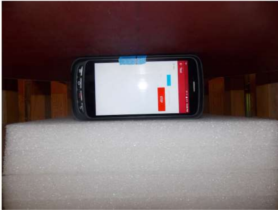
Test Position Left RFID Testing 0 mm Gap
