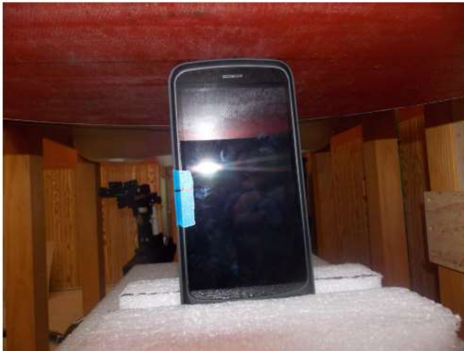
Test Position Top Testing 0 mm Gap
