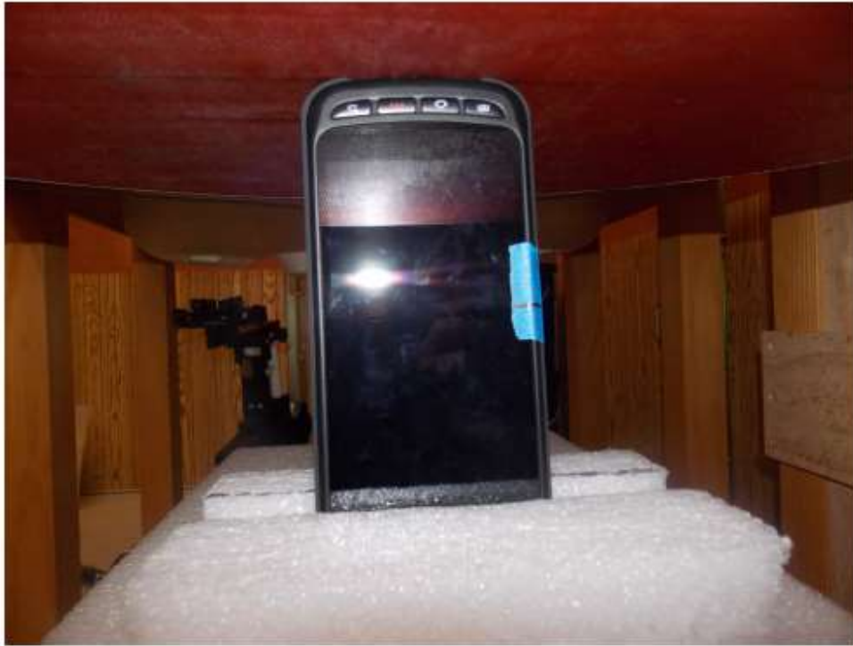
Test Position Bottom Testing 0 mm Gap
