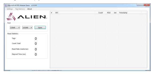
The window displays communication Port, Tag List and the Read Statistics information. Select the correct COM port and Open communication. The Engineering tab of the GUI will only appear when a module specific license is present in the GUI folder.
