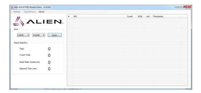
The window displays communication Port, Tag List and the Read Statistics information. Select the correct COM port and Open communication.
