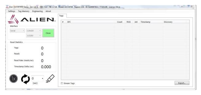
The GUI allows testing single inventory (1x) or timed testing. For timed testing type the number of seconds and into the window and hit the arrow. The test will run until the timer counts down to 0. Tags read by the Module will appear in the Right-hand window.
